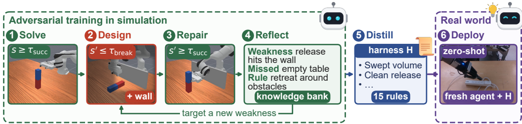
Figure 1: A 2 H overview. In simulation, a coding agent iteratively generates policies, adversarially designs task variations to expose failures, repairs policies, and reflects on the failures (1–4). The resulting experiences are distilled into a compact harness H (5), which guides a fresh agent in zero-shot policy generation for unseen real-world tasks (6).
